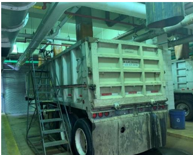
Figure 2-48 Open Bed Trailer Utilizing Three Discharge Points
