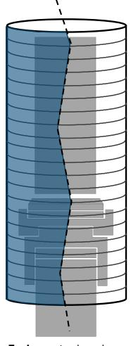
**Enclosure** to shroud the impact hammer
