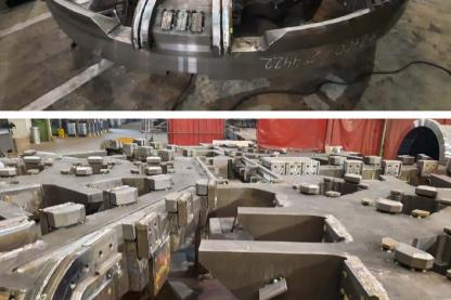
Tunnel Boring Machine Front Shield
