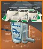
Tunnel Dewatering and Wet Weather Pumping Station
